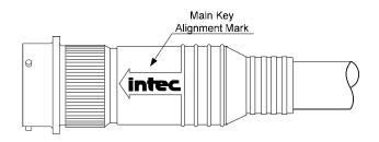
When making a connection, align the 5 keys on the connectors and turn the outer locking ring until locked. For XL cables with over molded back shells the arrow with the INTEC logo is inline with the main (top) alignment key.
