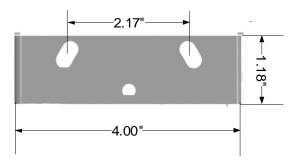
4. Once the holes are drilled, install the camera mounting bracket and extension, if required, with the mounting bolts provided. You may need to purchase additional hardware if the hardware provided does not work in your application.
